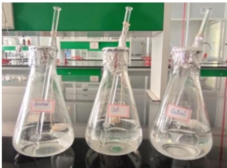
Figure 5: Calcium oxalate and inhibiting extracts enclosed in semipermeable and suspended in Tri's buffer
