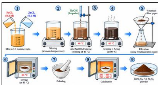
Fig.1 Schematic of \text{ZnFe}_2\text{O}_4/\alpha\text{-Fe}_2\text{O}_3 by nanoparticle synthesis by the co-precipitation method
