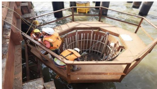
Figure: CHSL testing in offshore monopile
