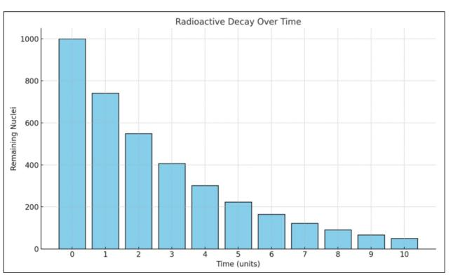
The column bar graph entitled Radioactive Decay Over Time shows visually (by the use of the graph diagram) the exponential decay of a radioactive component over a series of 10 time periods. The plot came out of the mathematical equation where n is the number of nuclei at the very beginning, and  $\lambda$  is the decay rate (Griggs, 2021). The number of the undecayed nuclei existing at a definite time interval, ranging from 0 to 10 units, corresponds to each bar.
