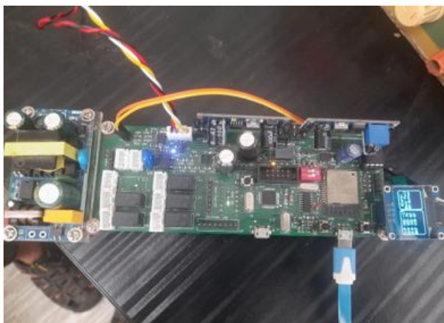
Figure 7: OLED of the HMI displaying real time values
