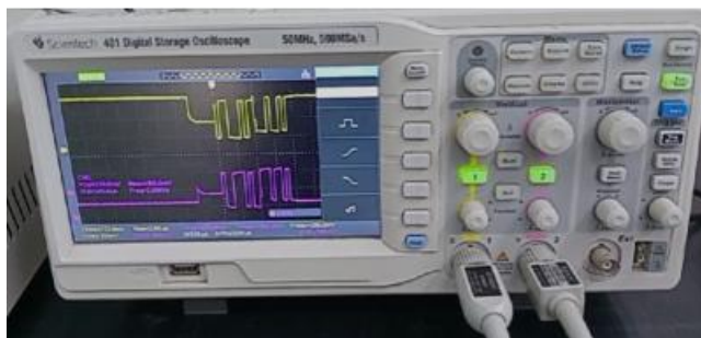
Figure 4: Real time data transmission and reception using RS485 protocol
