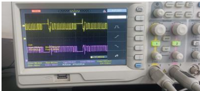
Figure 3: Real time data transmission and reception using CAN protocol
