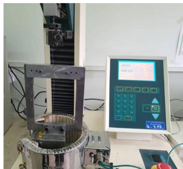
Figure 2: Attachment of the aluminum plate to the base of the Universal testing machine.
