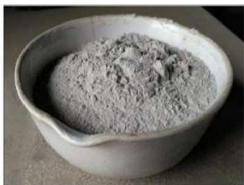
Figure 2.3: A photograph of ground granulated blast furnace slag Table Chemical properties of GGBS
