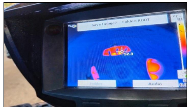
Figure 12: Thermal image of Front Brake Disc
