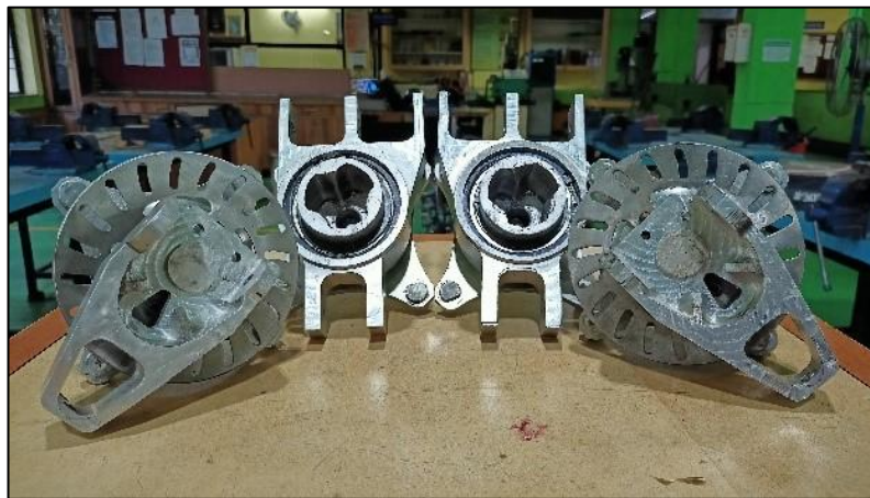
Figure 11: Front Wheel Assembly (Brake Disc with Knuckle)
