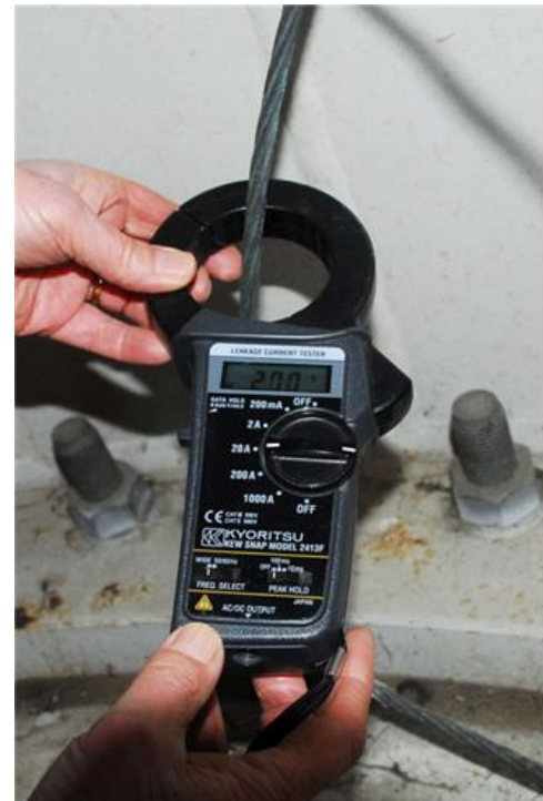
Figure 6: Measurement on one of the four separate grounding cables inside the wind turbine tower tube. The bolts are visible in the background.
