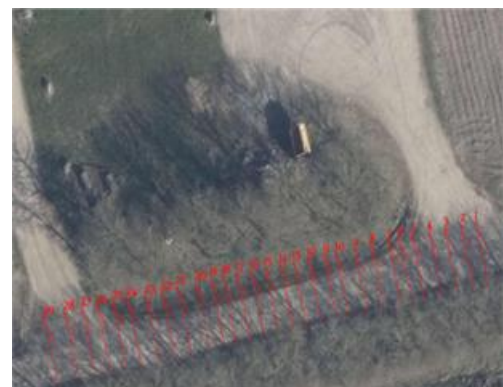
Figure 2: Positional mapping of 29 separate electrically conductive deposits. The dairy cattle barn is located north of the area in the aerial photo. A few hundred meters to the
