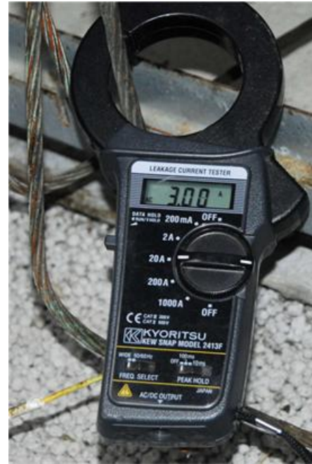
Figure 4: Verification measurements directly on one of the earthing cables from the transformer. Total calculated leak current from outside measurements was within 10% of the total current verified by direct measurement.
