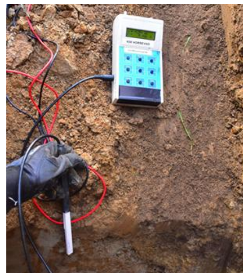
Figure 7: Magnetic Field measurement directly on a stray current carrying other deposit filament. The measured value of 135 \mu\text{T} and a distance of 5 centimeters correspond to a total current of 34 amperes.
