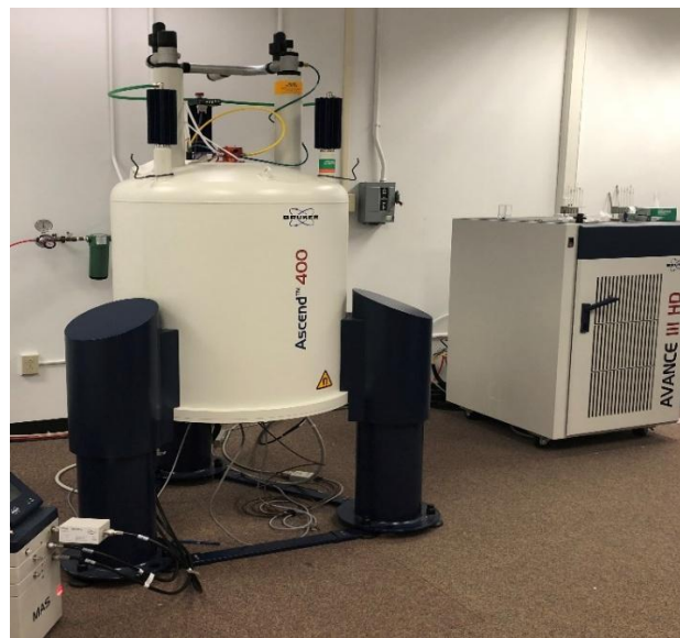
Figure 12: The 400 MHz NMR is equipped to collect data on liquid and solid samples using almost any NMR - active nuclei. https://chemistry.cas.lehigh.edu/facilities-menu/content/nmr-spectroscopy
