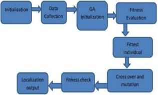
The block diagram illustrates the process of implementing Received Signal Strength (RSS) and Genetic Algorithm (GA) for node localization in a Wireless Sensor Network (WSN). Each step in the diagram represents a phase in optimizing node positions using RSS measurements along with GA optimization.
