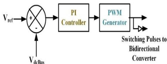
Figure 4: Battery Control
