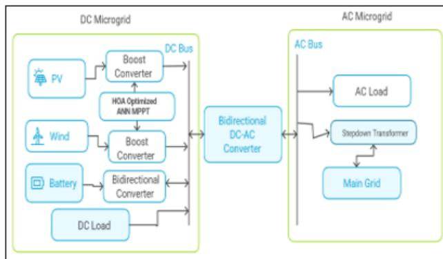
Figure 1: Proposed Hybrid Microgrid scheme
