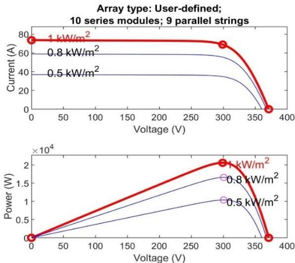
Figure 3: IV & PV Characteristics of PV
