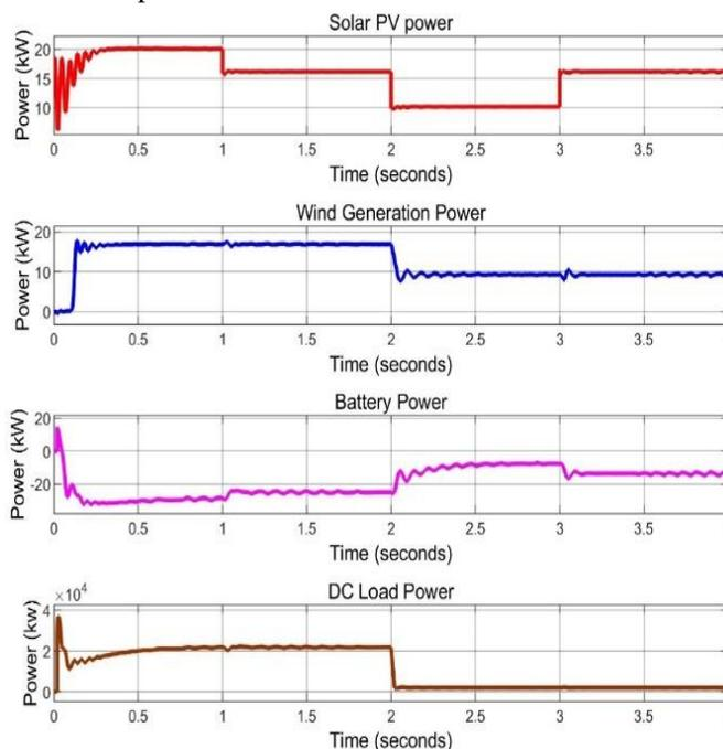
Figure 8: Powers of DC Microgrid
