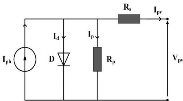
Figure 2: PV Equivalent Circuit
