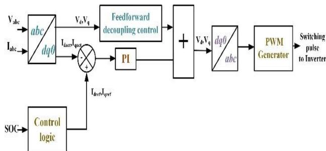
Figure 5: Control of Interlinking Converter
