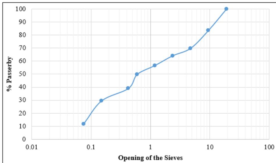
Figure 2: Granulometric analysis of the gravelly laterite from the Bafulato loan
