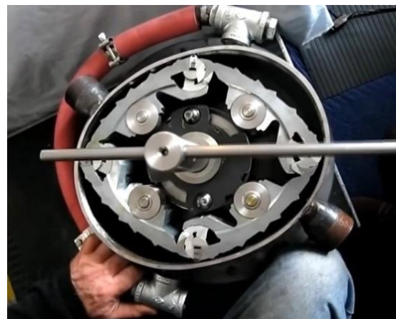
Figure 3: A look at the Quasiturbine (QT) technology? The Model QT-SC expander with internal Rotor and external Stator. The two intake ports are interconnected (red hose), and interlaced with opposed large diameter exhaust ports.
