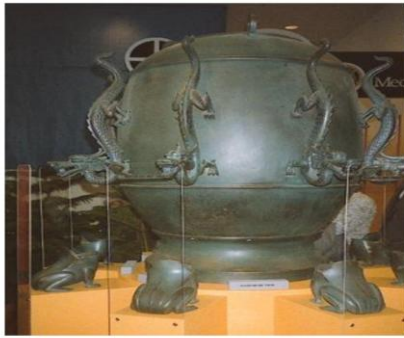
A large-scale model of Chang Heng's original earthquake weathercock.
