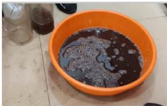
Black fluid drained from ICD-contains vegetable matter
