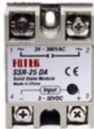
Figure 6: FOTEK SSR-25DA solid-state relays
