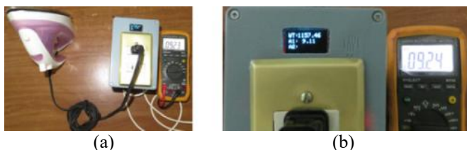
Figure 12: Iron usage: (a) Connection setup, (b) Current measurement
