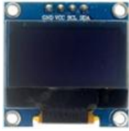
Figure 5: 0.96-inch I2C OLED display
