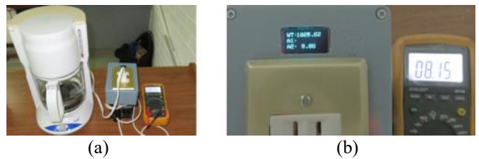
Figure 13: Coffee maker usage: (a) Connection setup, (b) Current measurement
