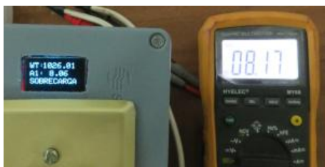
Figure 16. Overload Warning Displayed on the OLED Screen
