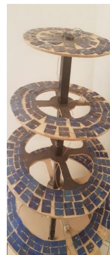
Figure 3: Photograph of the constructed solar tree prototype with a 64 cm × 64 cm base
