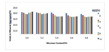
Void sin Mineral Aggregate for Bituminous Concrete Mixes at different PET Content Voids Filled with Bitumen for Bituminous Concrete Mixes
