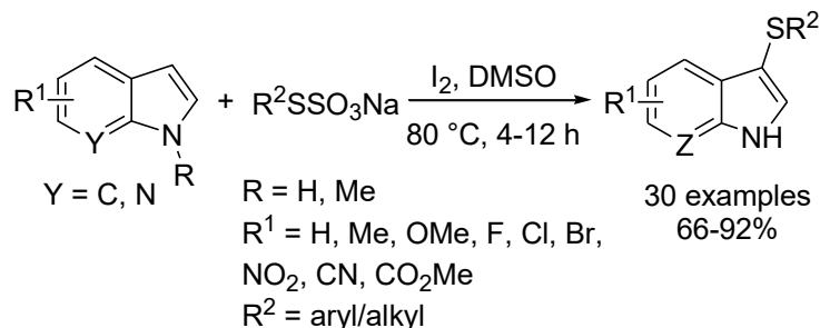
Scheme 2a: I 2 -catalyzed reaction of indoles with Bunte salts
