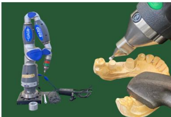
Figure 4: Measurement of cast using CMM
