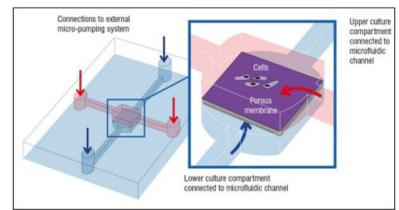
Visual representation of an OoC with microfluid channels and micro pumping systems to support cellular growth and functions.
