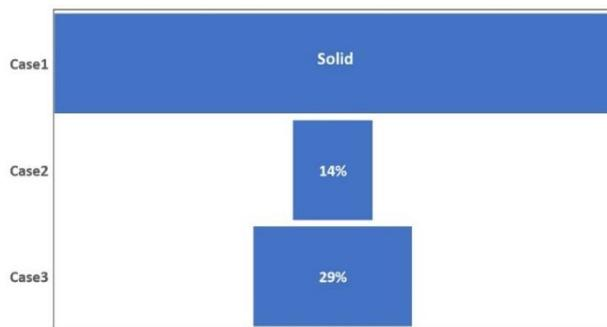
**Figure 4:** Mass reduction between solid and lattice structure ellipsoidal models
