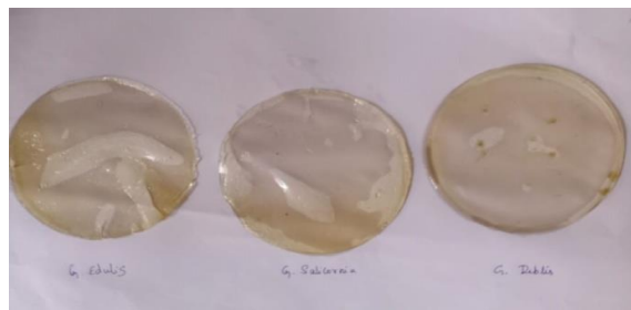
Figure 9: Bioplastic prepared from agar extracted from Gracilaria edulis, G. Salicornia and G. debilis
