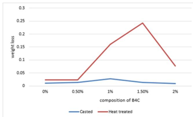
**Figure 8:** Weight loss comparison of untreated and heat treated at 20N.
