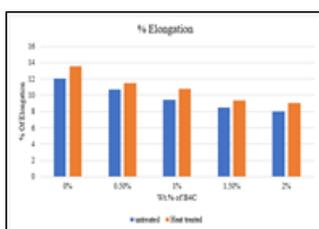
Figure 6: Percentage of elongation with increasing addition of Boron carbide
