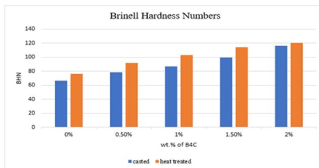
Figure 7: Hardness value of Al 7075-Mg-B4Ccomposites
