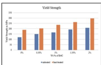
Figure 4: Yield stress with increasing addition of Boron carbide
