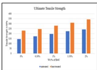
Figure 5: Tensile strength with increasing addition of Boron carbide
