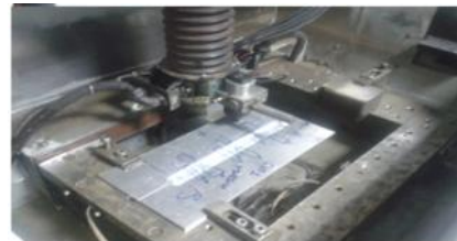
Figure 5: FSW Welding process
