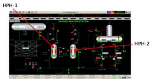
Figure 3.1: PLTU Teluk Sirih Preheater Installation Line (HPH)
