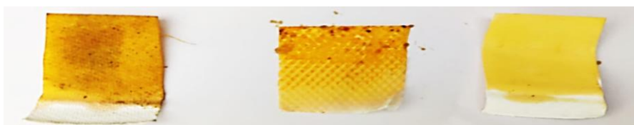
Figure 4: Shows the printing of the dye on to a) polyester, b) cotton and c) Silk
