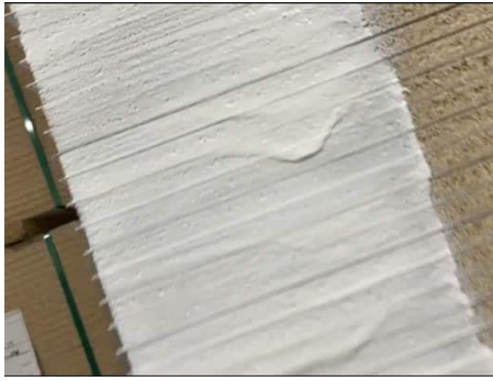
Figure 2: Defect detection – a thin or thick paint use case
