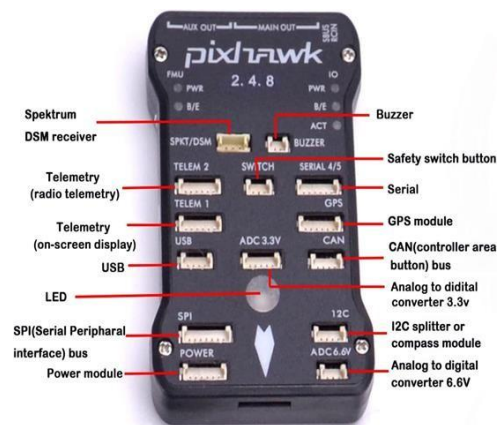
Figure 2: Pixhawk PX4 Flight Controller Pixhawk 2.4.8 32 Bit ARM CortexM4 high-performance processors Flight Control Board, Safety Switch, Buzzer, I2C Splitter Expand Module.
