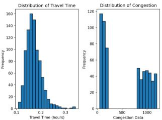
Most of the synthetic travel times are centred around a particular value, indicating a typical or average time travel time for the road segment. The histogram of congestion data on the other hand shows a skewed distribution, with a large gap and a tail extending to the right. Higher congestion values tend to be associated with longer travel times.
