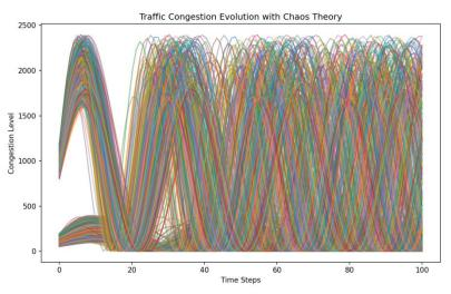
The simulation exhibits non-linear behaviour, as evident from the sinusoidal shape of the lines. This is because of the use of a non-linear functionto model the congestion dynamics. It demonstrates how small variations in traffic volume and speed can lead to significantly different congestion levels over time.
