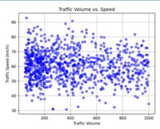
Clearly, it is seen that traffic speed and traffic volume have no clear pattern and are heavily scattered. There is an apparent concentration at low volume and speed of around 60 kmph, where 60 kmph was defined as the mean speed and volume changes based on time of days. The heavily scattered and no clear pattern in traffic volume and speed indicate the complex and dynamic nature of traffic flow.
