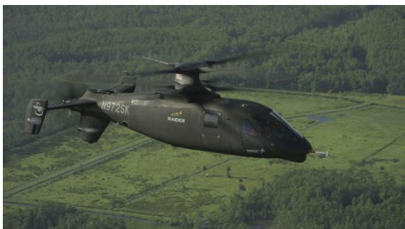
Sikorsky S - 97 Raider conducts flight tests, demonstrating its high - speed and agile capabilities.
