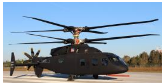
Sikorsky - Boeing SB>1 Defiant during a flight test, showcasing its coaxial rotor system and pusher propeller. Image source: Breaking Defense
