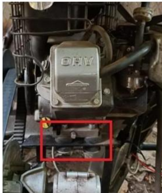
Figure 9: Rubber Bushes for NVH Consideration
