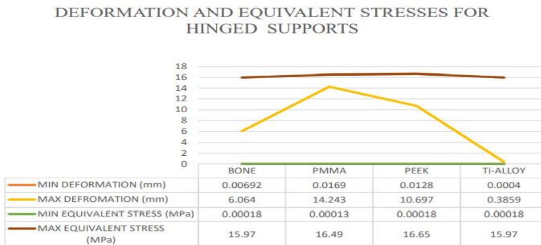
Graph 2: Deformation and Equivalent stress for different materials under Hinged end conditions
