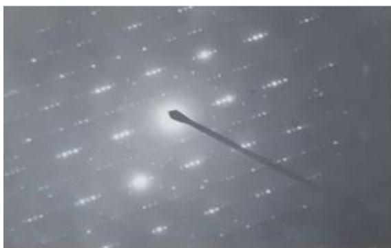
Figure 10: Depict the electron Diffraction pattern of Sample No. 3
