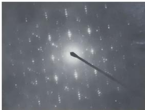
Figure 7: Depicts the Electron Diffraction Pattern from overlapping crystals
