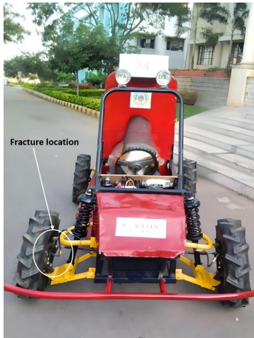
Figure 10: Failure Location of the ATV during Final Race Event
