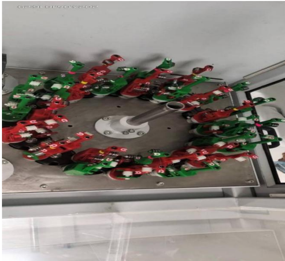
Figure 1: (A) Carriers are Mounted onto a Braiding Machine, where the Braiding takes place
