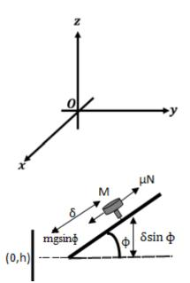
$\phi$  is the angle made by the platter with x axis. h is the height from the ground. M is the mass of the spinner
