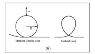
When a roller coaster enters the loop - the - loop, it is travelling at a high speed and must maintain enough speed and momentum to complete the loop without losing velocity. As the coaster continues to travel through the loop, the angle of descent gradually decreases until the coaster reaches the end of the loop and returns to an upright position. There are four primary forces acting on a roller coaster as it travels through a loop - the - loop:
