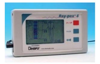
Bingo 1020/Raypex (Forum Engineering technologies, Israel) said to be a fourth generation device. This unit uses two separate frequencies 400 Hz and 8 KHz similar to the current 3<sup>rd</sup> generation unit.<sup>19</sup>
