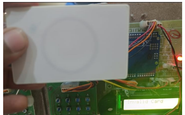
Figure 11: Scanning of invalid RFID card
