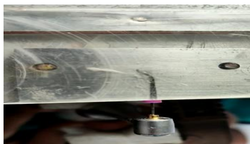
Figure 2: File rotated in the groove in static mode until fracture
