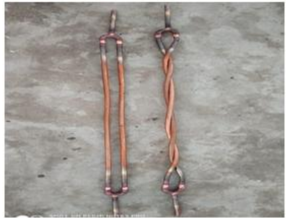
Plate 7: Assembly of Straight and Twisted Pipe
