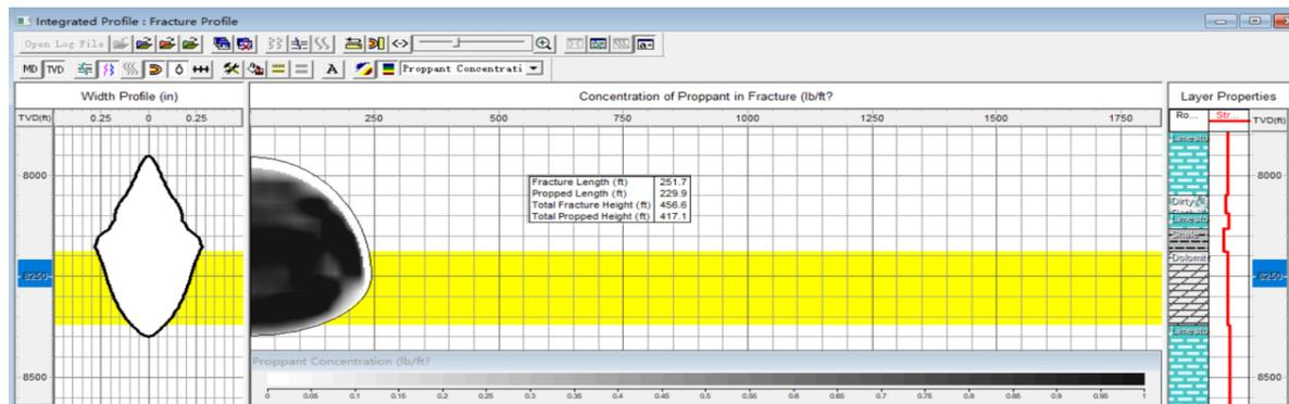
Figure 2.1: Comprehensive cross - section of the crack model
