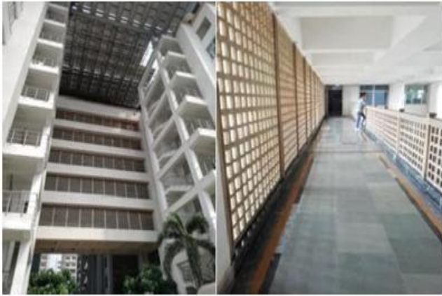
Figure 3.9: Cross ventilation through jaalis (Source: Author)
