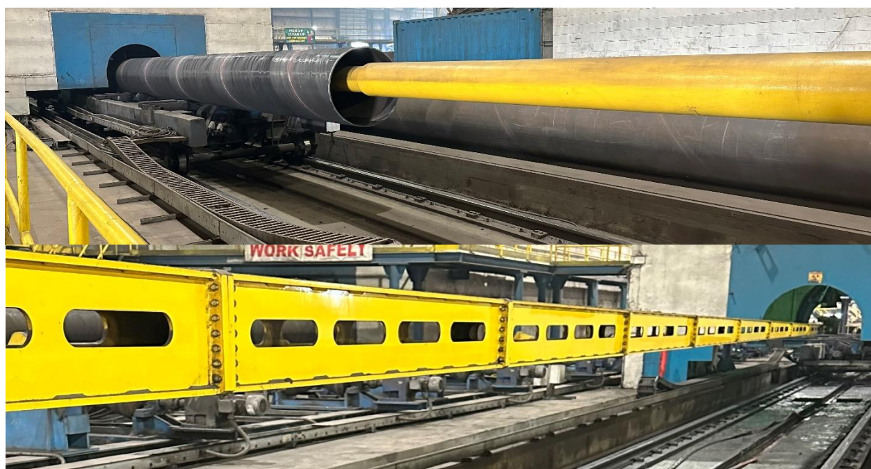
Figure: An example of a boom (for installation base of flat panel or X - ray tube) with wagon for pipe transport
