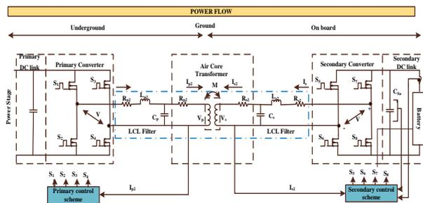
**Figure 8:** Bidirectionally IPT setup with binary active ground layout. Active rectifying allows draw - in vehicles and V2G functioning [41].
