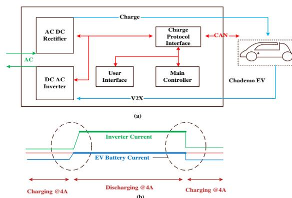
Figure 2: The setup used for V2G and dynamically charging with chademo v1.2 (a) and EV current & its voltage waves (b) are shown in Fig.2. Chademo's charger & EV are linked via a CAN bus connection.
