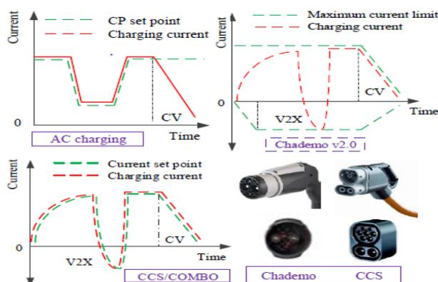
Figure 1: Dynamic charging using AC, Chademo v1.2 and CCS/COMBO
