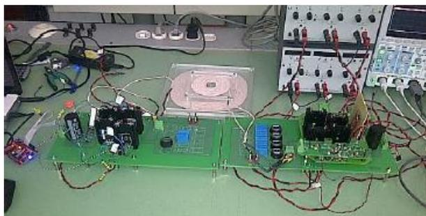
**Figure 9:** Lab - scale bidirectional IPT setup [42].
