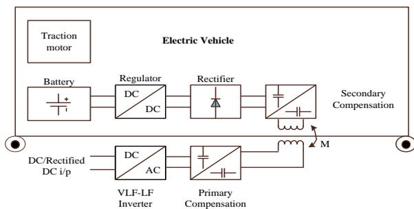
Figure 6: EV IPT grounded system for power conversion stages
