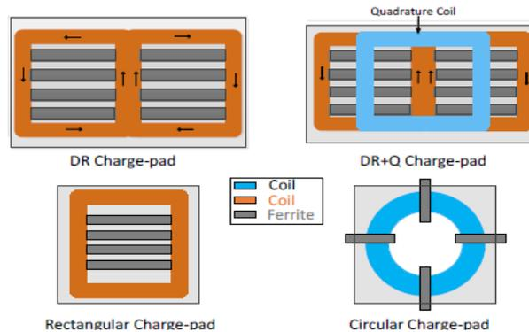
Figure 7: Multi - coil and single - coil charging pads. The Quadrature (Q) coil catches perpendicular flux and the DR vertically flux. [38]
