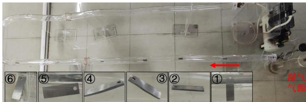
**Figure 1:** Visualization of wet gas pipeline simulation device
