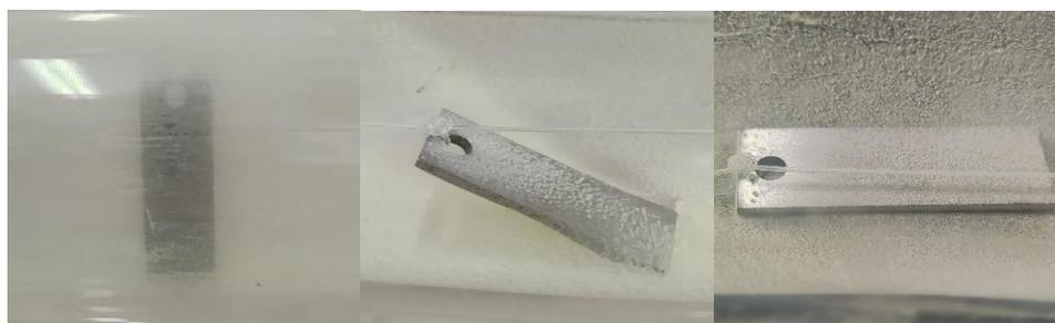
Figure 2: Suspension and deposition state of elemental sulfur
