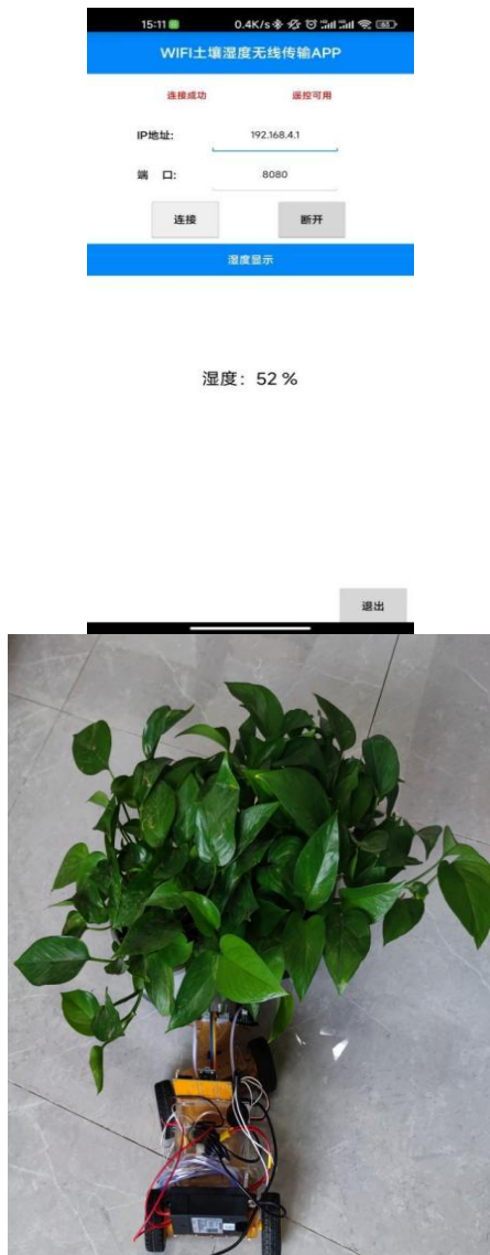
Figure 10: Display figure of soil numerical monitoring of mobile phone APP
