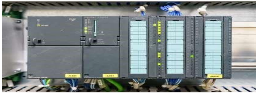
Figure 1.12: Siemens industrial programmable logic controller.
